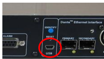
Figure 2 Front panel USB connector
